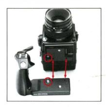
C. Place the camera main body on the base of the Speed Grip G, with the guide pins on the accessory aligned to the accessory mounting guide sockets on the camera base, as well as meshing the winding couplers on the accessory and camera base.
