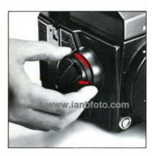
A. Detach the film winding crank from the camera main body. Pull the release lever on the base of the film winding crank assembly outwards and, at the same time, rotate the base in the counter-clockwise direction until the assembly comes off.
