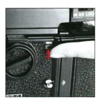
B. The shutter release buttons are locked against accidental use, by pushing up (OFF) the main switch on the camera main body.
