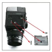
B. Take off the cover of the base, winding coupler and flash synch contact from the base of the camera mian body.
