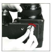
D. Finally, tighten the attachment screw on the base of the accessory and connect the two together securely.
